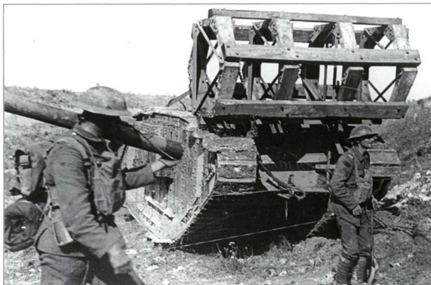
The crib, essentially a lighter, reusable fascine, was rarely seen on Mark IV tanks, but this female with a broken track is carrying one during the attack on the Hindenburg Line on 27 September 1918 in support of the Canadians.
