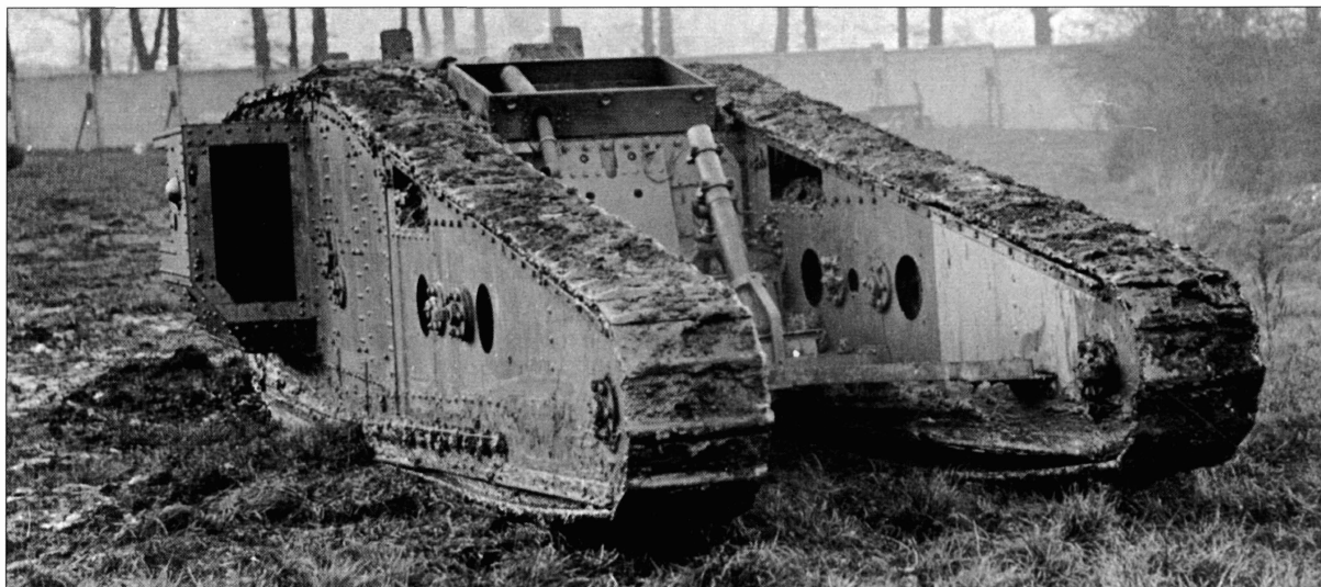
The Mark IV male Tadpole Tail, posed at Dollis Hill to display its rear extensions and a 6-in. mortar mounted to fire over the tank. Tests were also carried out on firing mortars from inside male sponsons.
