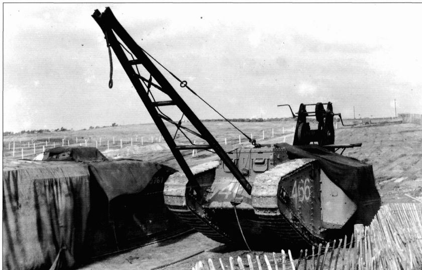
Number 466 was the unusual combination of a training tank with supply sponsons. It was used at Bovington as a crane tank with a standard jib. The big winch at the back operates the hoist instead of the usual chain system.
