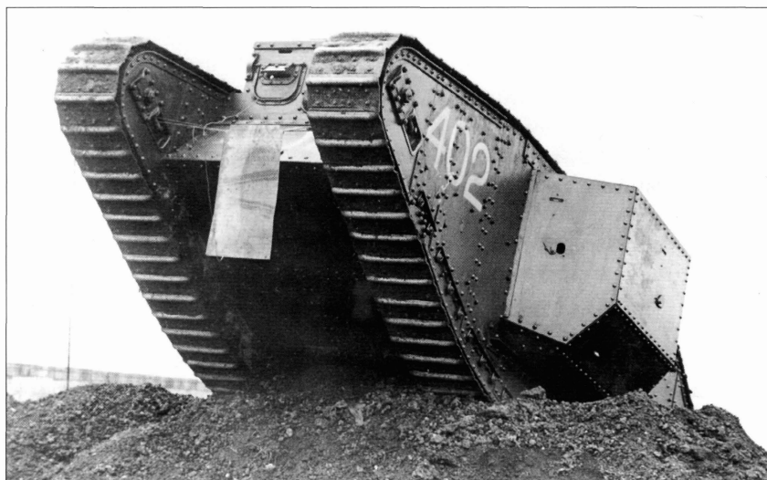
This is the Mark IV supply tank used for aircraft-to-tank wireless communication trials at Biggin Hill towards the end of the war. The panel suspended by string between the front horns is presumably something to do with the receiving process.
